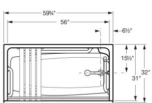
FEATURES Dimensional Tolerance ± 1/4". Dimensions needed for site preparation should be measured from the unit. American Bath Group assumes no responsibility for preparatory work.
