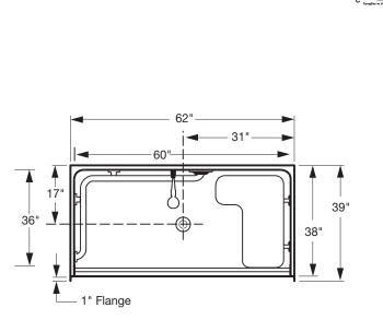
FEATURES Dimensional Tolerance ± ¼". Dimensions needed for site preparation should be measured from the unit. American Bath Group assumes no responsibility for preparatory work.
