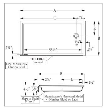
One piece, single threshold model for recessed installation. Features 1" flange on three remaining sides. End drain.
