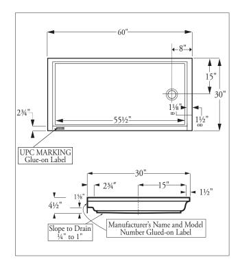
Dimensions may vary  $\pm 1/4"$  inch. Please check unit before installation. Place receptor on a bed of mortar or plaster for warranty compliance.
